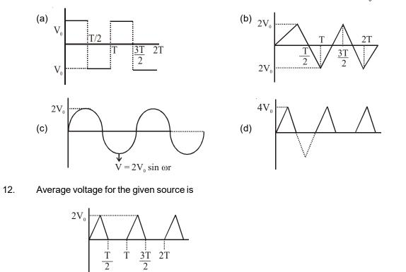
11. Current time graph of different source is given which one will have R.M.S. value  $V_0$
